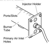
Figure 35 - Injector Holder On Outlet Burner Tube
